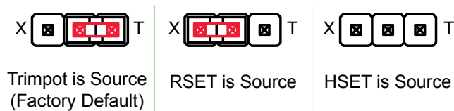
Figure 7. VSET Source Jumper Settings
